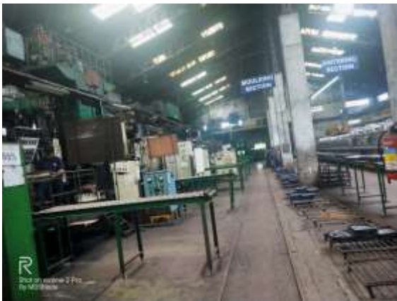
Molding Section for forming the magnetic cores for different applications (Dry Process)
